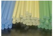
**TECAPEEK™ MT**: Colored rod produced from VICTREX® PEEK™ 450 resin. Current colors available are yellow, green, blue and black. All pigments are organic based and FDA compliant. TECAPEEK™ MT is tested to USP Class VI on an annual audit basis and is intended for medical instrumentation and orthopedic sizing trials. Most colors are stocked domestically in 12 and 25 mm rod. Other rod diameters are available on a custom production basis.
